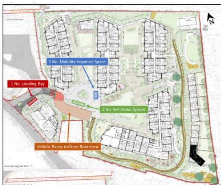
Figure 3.1: Podium Level Parking Spaces
